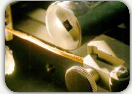
STRETCHING APPARATUS INSTALLED ON THE SAXS BEAMLINE OF THE AUSTRALASIAN SYNCHROTRON
