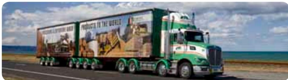
This large two trailer truck had its initial road test in late December. Although the low speed turning performance characteristics of the vehicle had previously been calculated by Transport Engineering Research New Zealand (TERNZ) using a computer simulation model, the road controlling authorities required a physical test on the route that the vehicle will be using. "The vehicle's performance was very close to its predicted performance and it was able to travel its route between
