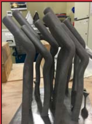
Printing for Team NZ Cycling; lightweight titanium handlebar extensions.
